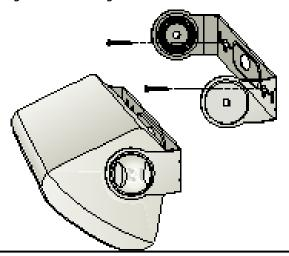
NEVER use pliers or power tools to tighten the knobs.
